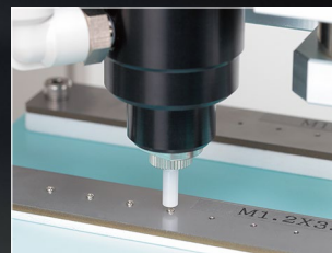
Tightens screws as small as M1.0.
